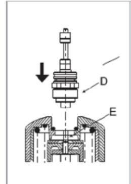
Place drive bar D into the drive and screw threaded lock A onto drive lever E.
