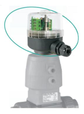
Direct return valve positioner can be rotated 360 ° directly installed on the valve, the valve position and its status can be reported to the upper system by Electric remote report. The built-in LED light emits optical position feedback.
