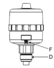
Install the return sensor housing to the drive rod D, rotate the sensor housing, set the direction of the cable glands, and ensure that the electric shock signal is normal. Use the Allen wrench to tighten the fixing screw F
