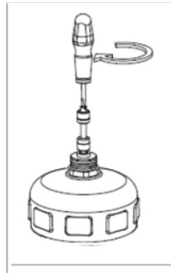
Tighten the drive rod and driver rod with a driver
