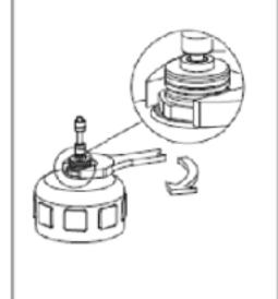
Use a wrench to tighten the drive rod to the top of the drive
